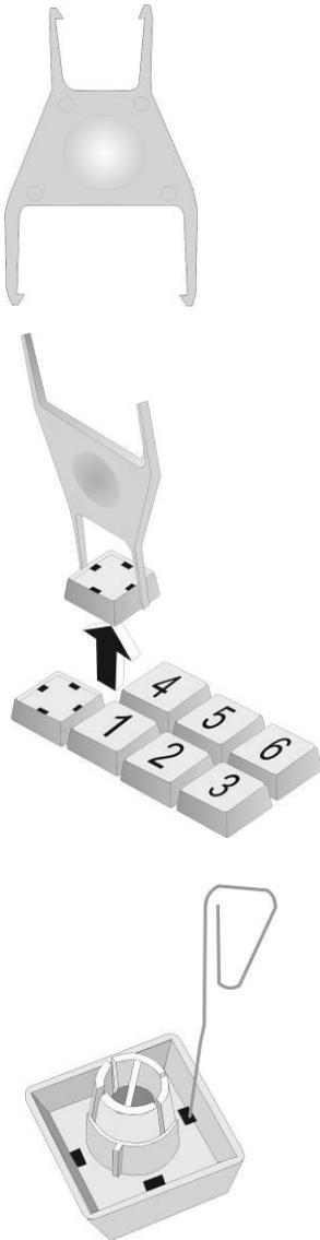
You can remove each of the key caps using the key removal device enclosed, pulling the key upwards.
