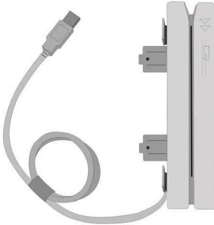
The swipe card reader (MSR Module), that is available as an option, can read three ISO tracks simultaneously in a single swipe.
